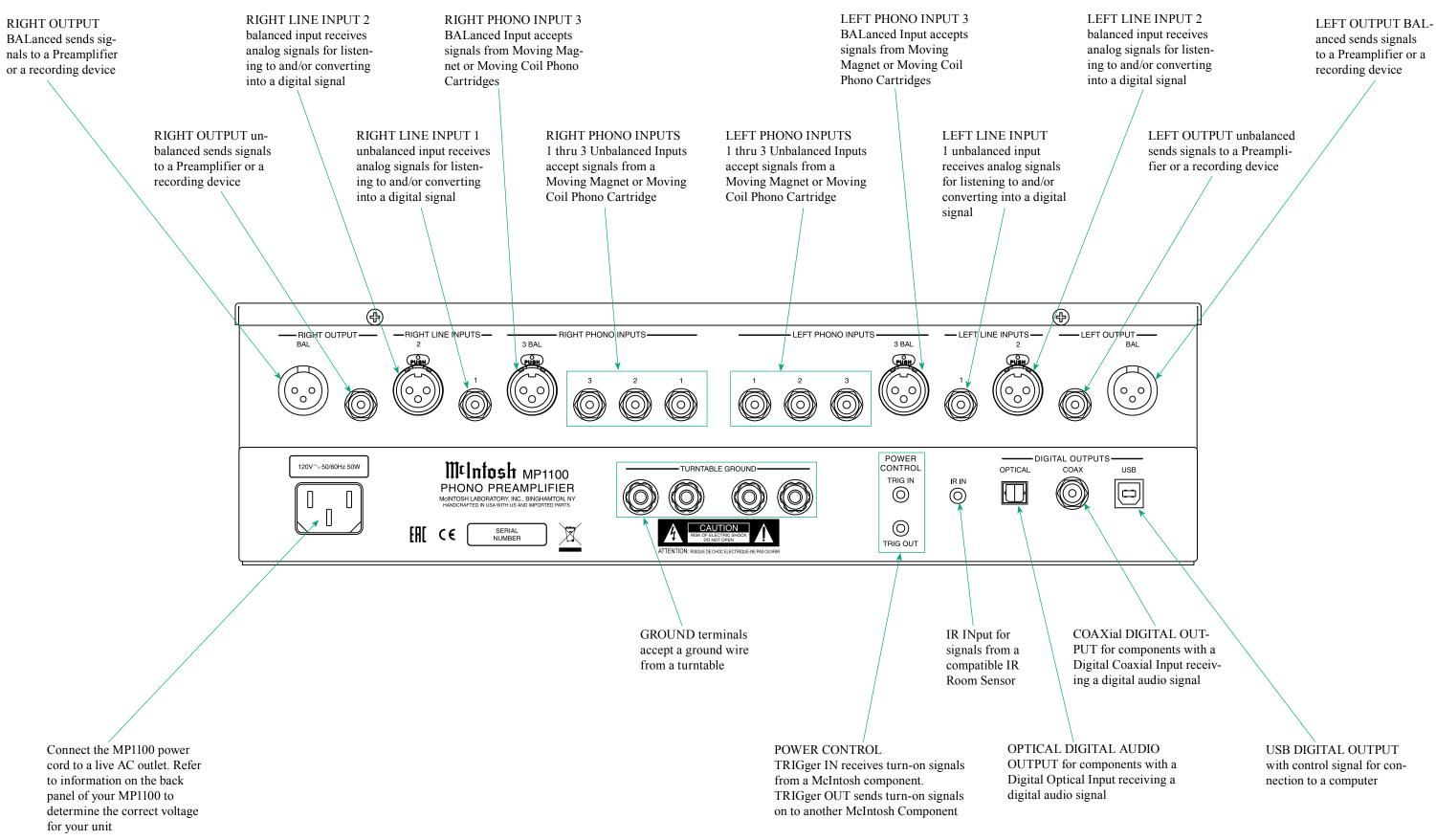
USB DIGITAL OUTPUT with control signal for connection to a computer
